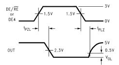
Figure 8. Driver Enable and Disable Timing (t<sub>PZL</sub>, t<sub>PLZ</sub>)
