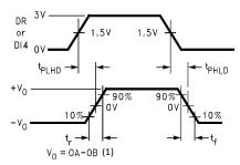
(1) Differential propagation delays are calculated from single-ended propagation delays measured from driver input to the 20% and 80% levels on the driver outputs (Figure 16).
