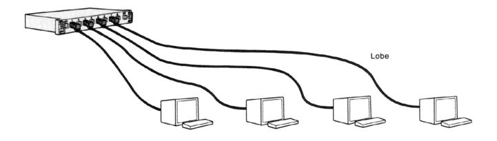
IBM 8228s can be linked together to form rings that are larger than eight lobes by attaching the RO receptacle of one 8228 to the RI receptacle of another 8228, as shown below.
