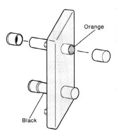
This device is used to adapt the distribution panel connector slots for use with optical fiber cable biconic connectors rather than the standard IBM Cabling System Data Connector. It is also used with the strain-relief mounting bracket supplied with the surface-mounting assembly.
