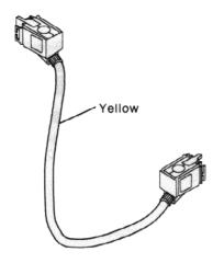
The crossover patch cable is a specially designed cable used with two 8218s, 8219s, or 8220s to provide repeating capability for the backup path. Crossover patch cables are not required for use with IBM 8230s. The crossover patch cable is 2.4 m (8 ft) long. The cables are yellow to distinguish them from ordinary (black) patch cables. Crossover patch cables cannot be repaired in the field. Chapter 3 of this manual describes use of the crossover patch cables with 8218s, 8219s, and 8220s.
