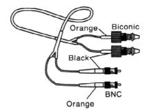
These specially designed patch cables are used to connect the 8219, 8220, or 8230 to any multimode optical fiber cable terminated at a distribution panel or at a strain-relief mounting bracket using biconic connectors. The cable is 2.4 m (8 ft) long. The ends of the cables that attach to the 8219. 8220, or 8230 are color-coded with black and orange heat-shrink tubing to distinguish the two optical fibers in the cable.
