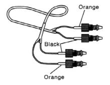
These patch cables are used to connect any two pieces of multimode optical fiber cables terminated at a distribution panel with biconic connectors. These cables are available in two lengths: 2.4 m (8 ft) and 9 m (30 ft). The connectors are color-coded orange and black to distinguish between the two optical fibers in the cable.
